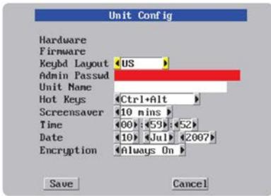
Selecting the Unit Configuration allows you to define the Unit setup details such as the keyboard layout, admin password, time and date, and encryption.
