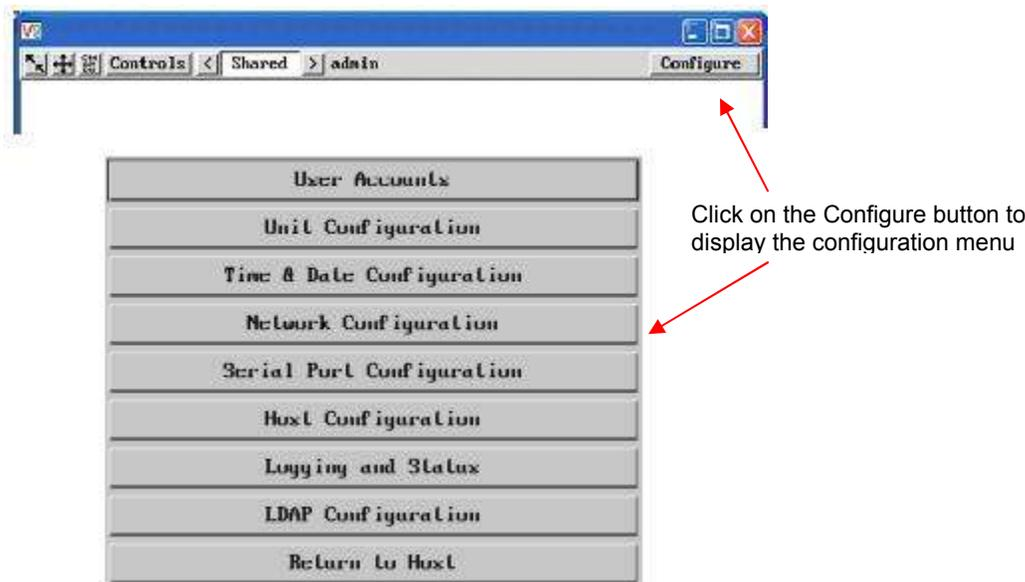
Figure 13. Accessing UL2-DVI Configuration
