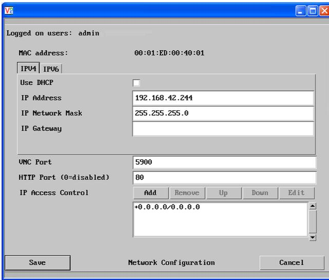
Figure 14. Setting Initial IPv4 network address
