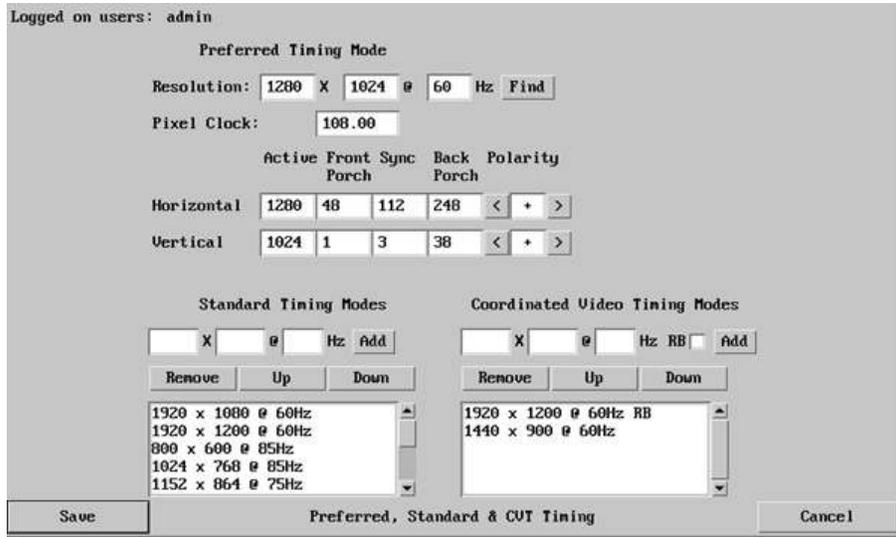
Figure 53. Preferred, Standard & CVT Timing Screen
