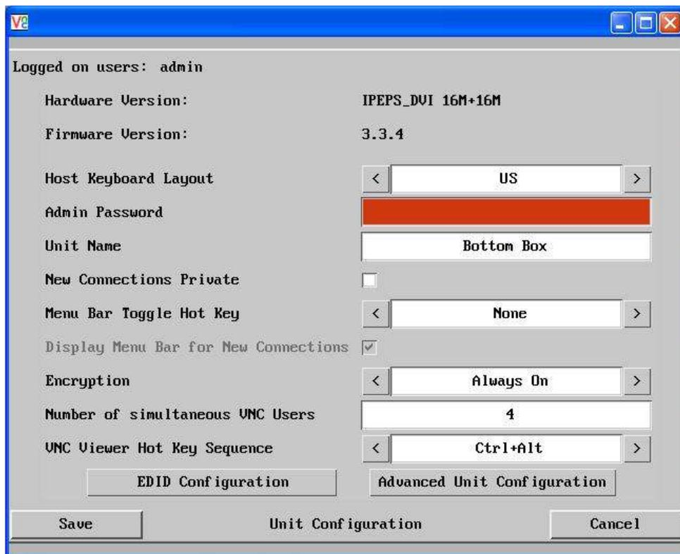
Figure 51. Unit Configuration Screen
