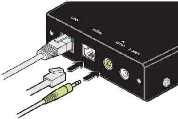
Figure 6. Optional Serial and Audio connections
