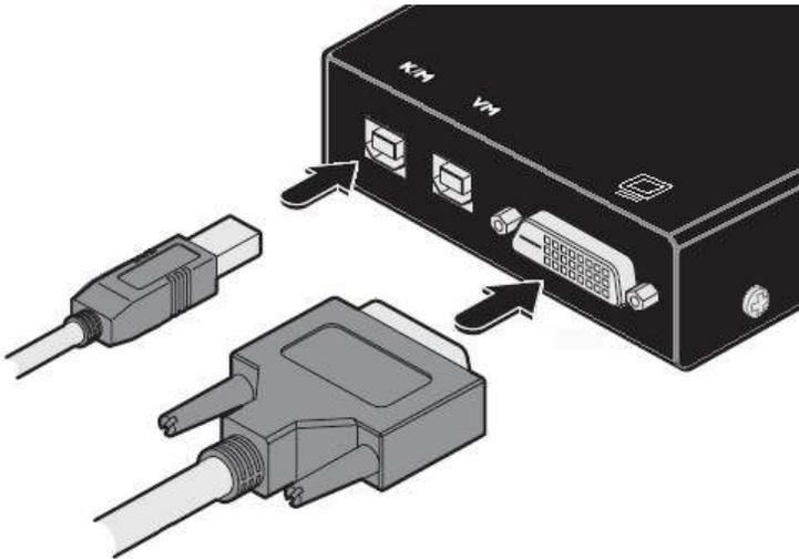
Figure 4. Keyboard/Mouse and DVI connections
